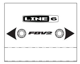
The FBV2 functions as a two button channel scroll foot switch. This foot switch allows you to scroll through the 4 channels (the A,B,C & D buttons) of your Spider Valve.
