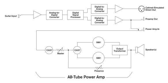
As you can see, Spider Valve consists of a complete Class AB tube amplifier fed by a digital front end, which houses all the magic of our amp and effect models. Make no mistake; these are not "marketing tubes". This is a real tube amp. 12AX7 pre-amp tubes, which are always working to provide the harmonic richness and compression of a great vintage tube amp, drive the phase splitter and 5881 power amp complement.
