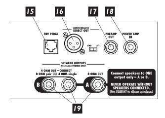
**FBV Pedal** – Plug in one of our optional Line 6 FBV foot controllers for channel switching, tap tempo, effects on/off control, wah/volume pedals, access to 32 more channel memories, and tuner capabilities. See Chapter 4 for more details.
